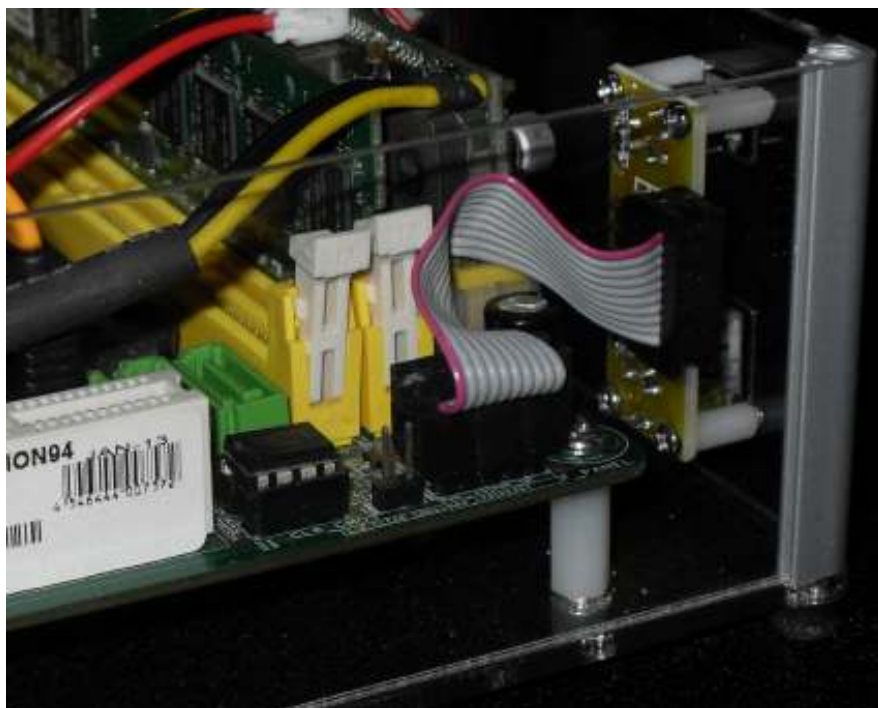
2.11 Connecting internal USB cable of front panel LCD to USB connector of motherboard
