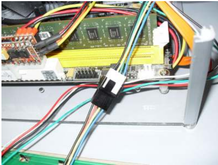
2.12 Connecting the 2-way PWM fan cable (4-cable one for detecting the CPU fan speed) to CPU fan
