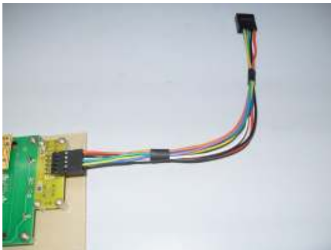
2.8 Connecting ON/OFF switch cable to front panel
